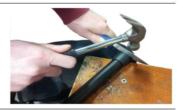
A small piece of the plastic stud will remain in the plastic cup. Remove this on all three plastic cups by using a hammer and a screw driver or center punch.
