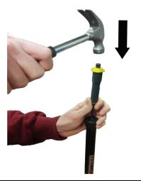
3. When attaching the new seat, use a rubber hammer to attach the plastic studs to the plastic cups. Verify that the plastic stud and seat is properly fixed by pulling the seat near each corner.
